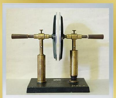
A simple demonstration of a parallel-plate capacitor
