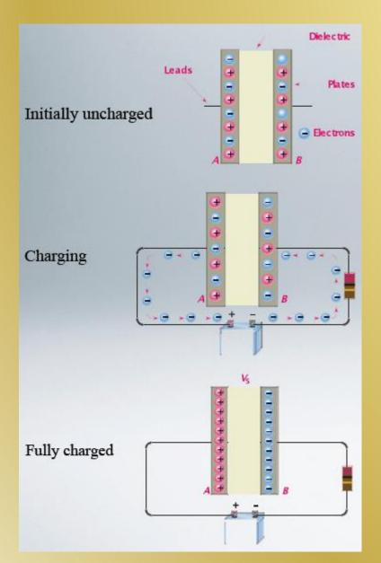
A *capacitor* consists of a pair of conductors separated by a dielectric (insulator).
