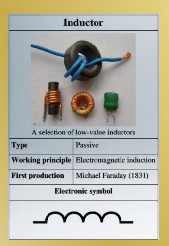
An inductor is a two terminal element consisting of a winding of N turns capable of storing energy in the form of a magnetic field
