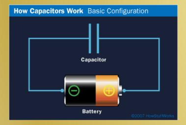
The capacitor plate attached to the **negative terminal** accepts **electrons** from the battery.
