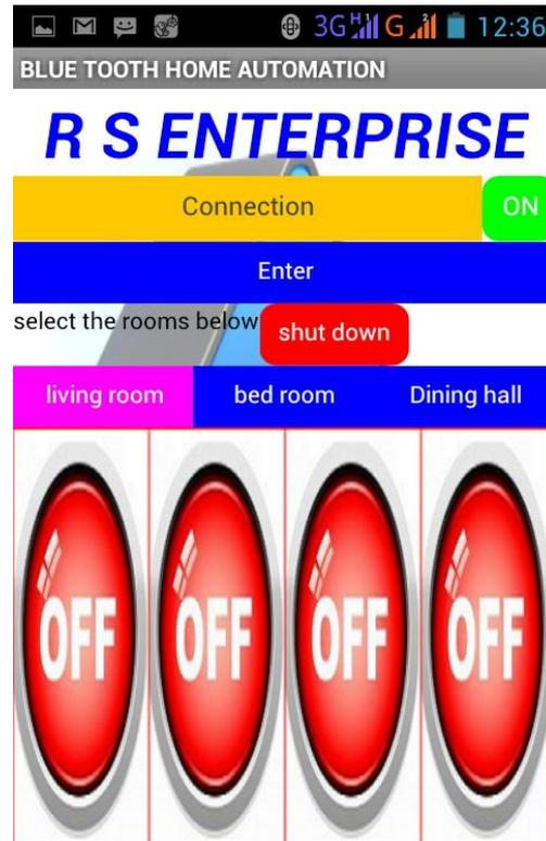
**STEP 7: Select the connected devices which you want to control by clicking the OFF option it is converted to ON {See below} FOR EX: if your connected devices is tube light in the living room it will started glowing**
