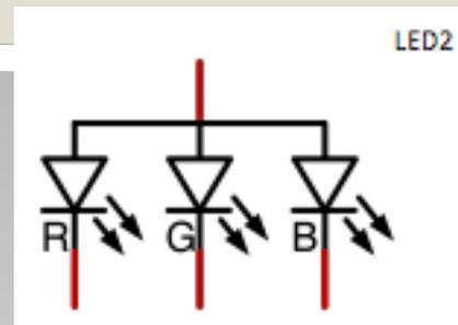
Try resistors out in various combination to make different colors. Experiment by adding potentiometers to the leads.
