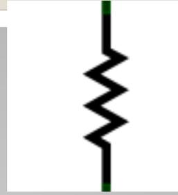
Resistors provide a specific amount of resistance to a path in a circuit or wire. Ohm's law is used to calculate the properties related to resistance.
