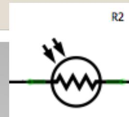
Photoresistors change their resistance by the amount of light detected.
